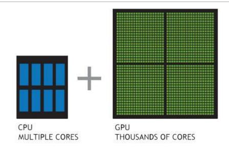
**GPUs** have thousands of cores to process parallel workloads efficiently
